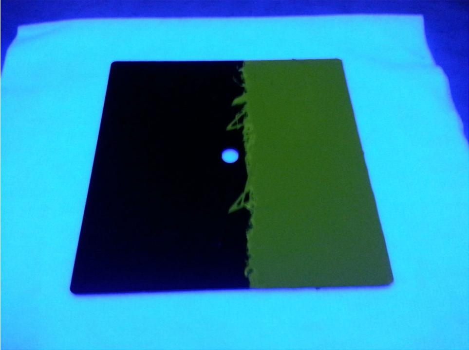
The following picture shows the mask line after the masking has been removed, how the clean edge is formed between the masking and the anodized
